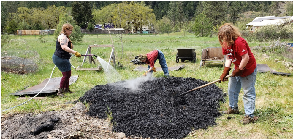
Quenching the biochar: spray and rake it thin so it loses heat.
