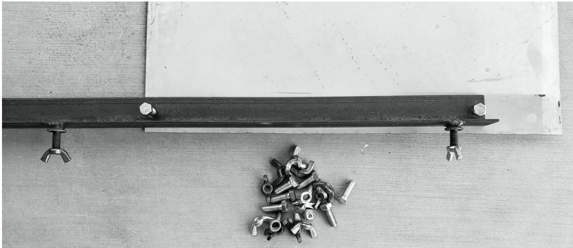
The Connector Bracket showing the arrangement for attaching the Heat Shield. The Heat Shield extends 4 inches above the top of the Kiln Body.
