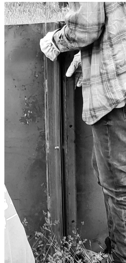
The Connector Bracket showing the arrangement for attaching the Heat Shield. The Heat Shield extends 4 inches above the top of the Kiln Body.
