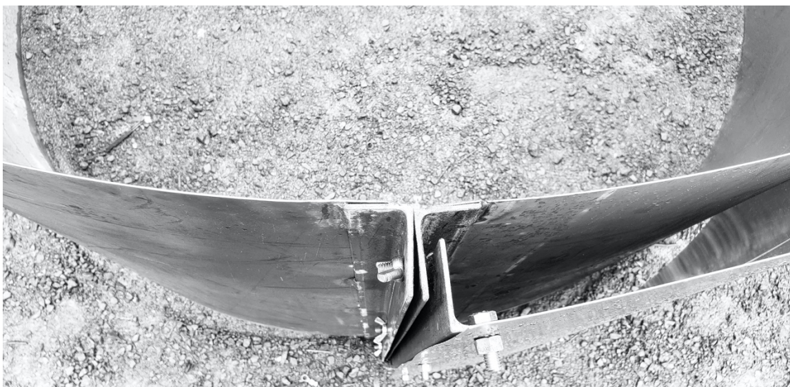
Partially assembled kiln showing the bracket that holds the Kiln Body sheets together and provides a means of attaching the heat shield.
