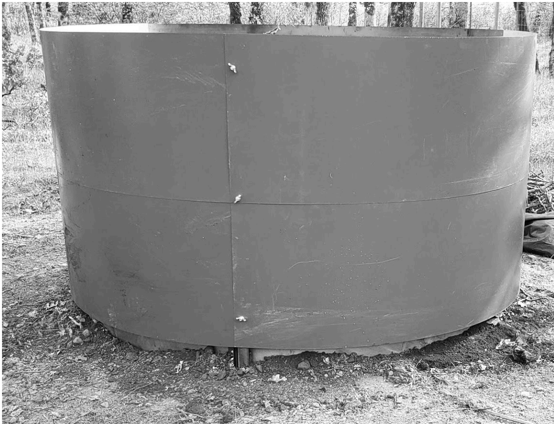
Completely assembled kiln. Notice that the kiln bottom has been sealed by pushing up dirt around the bottom edge.
